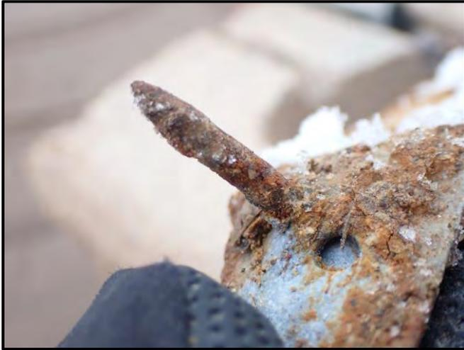
Figure 22: Corroded PAF
